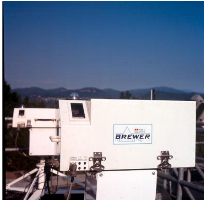
Figure 1. Single (back) and Double (front) Brewer spectroradiometer, both pointing East
