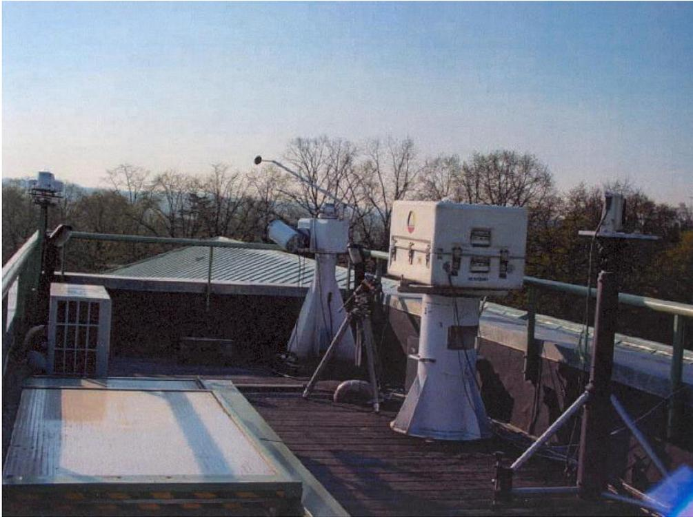
**Figure 1. View from roof platform, looking South-East (spectroradiometer in middle-ground; pyranometer with shadowband & SPUV-10 filter radiometer in background)**
